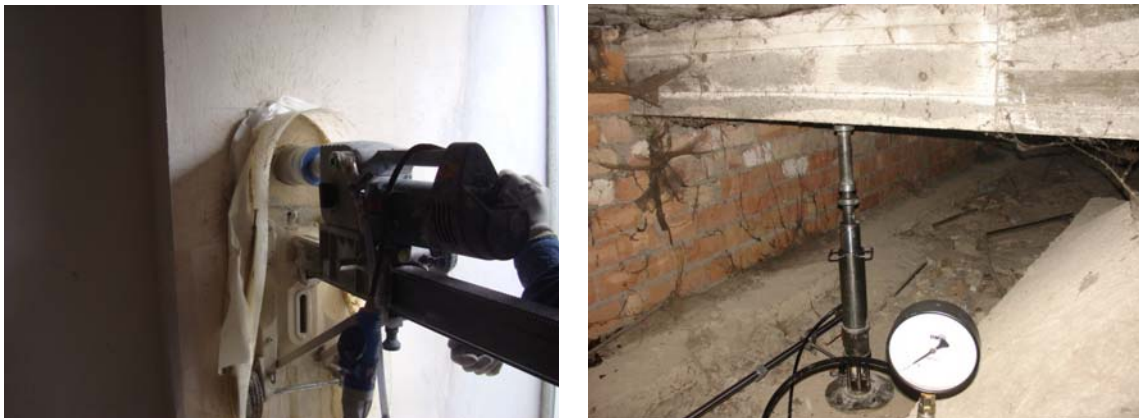
Figure 1: carrots machine in action, and test of load on plates
